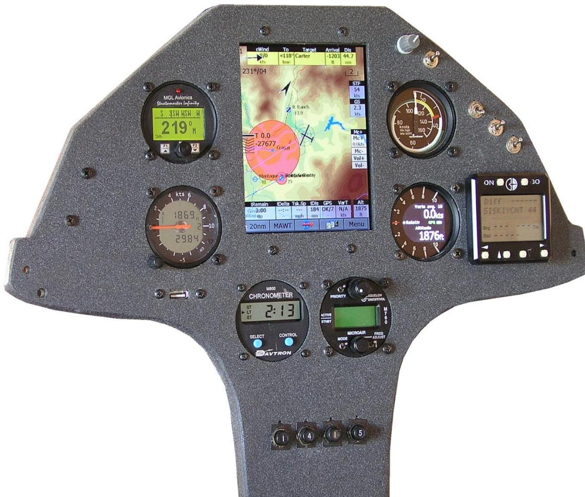
SailPlane Cockpits are enhanced by Craggy Aero's Ultimate Le Flight Computer. The System is a modular design and can use the hardware and software familiar to soaring pilots. Designed specifically for sailplane panels, you can use current hardware or grow your system as your needs and budget dictate. Pilots can start with an Ultimate Le and a NMEA GPS source or build an integrated system with Variometers, IGC logger, and PowerFlarm.
