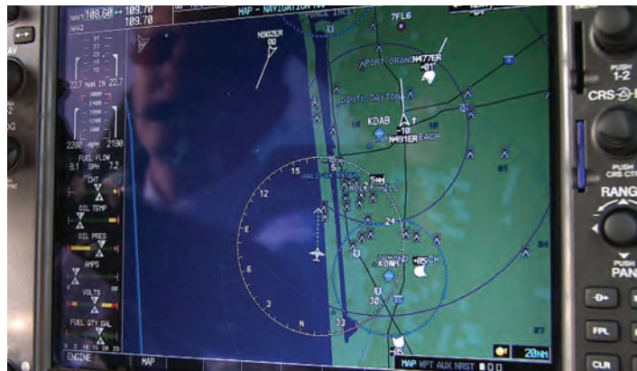
Pilots equipped for ADS-B In can see the positions of other aircraft reported by ADS-B Out and radar on a cockpit display.
