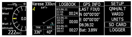
As a data transfer medium serves a micro size **SD card** and this makes possible to provide all data inputs and also downloading of flights after using of SD card. The Colibri II stores flight data into its internal memory, so operation **without SD card inserted** doesn't mean loosing of any flight data.
