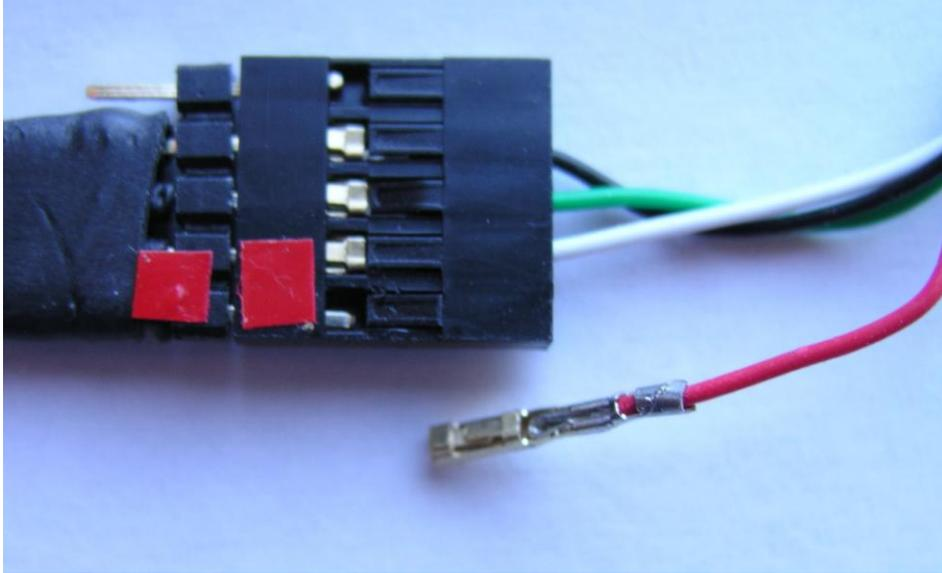
A connector is provided for sticks that have a small access hole for wires. Remove the wires and thread thru the stick. Pay close attention to how the wires are secured into the connector. You can lift the plastic tab and pull out the contacts. Push tap down before reinserting the contacts. Insure the wires are in the correct color order. Red, white, green, black.
