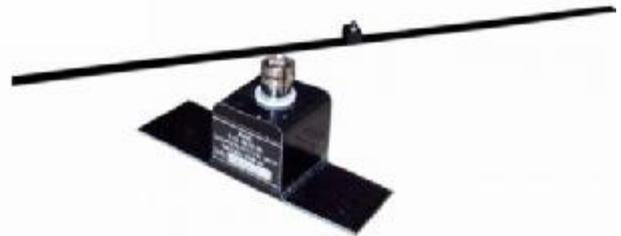
Base station antennas - usually longer in length than standard  $\frac{1}{4}$  wave antennas, most base station antennas are  $\frac{1}{2}$  wavelengths being approximately 1.2 m long plus a base section. They are normally 'ground plane independent' (meaning that the ground plane is 'in-built') and are mounted vertically on towers or the side of buildings. They are of course not suitable for flying (unless you want to loose 30 knots).
