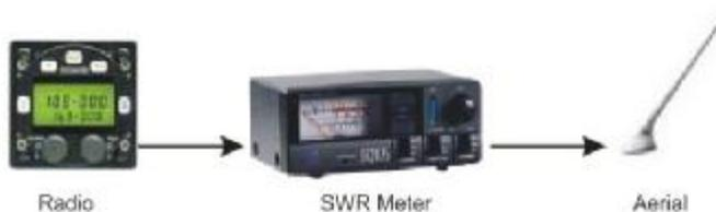
Rig the aircraft and move it well away from hangars (and hangers-on for that matter). SWR'ing inside a hanger is a complete waste of time because the meter will measure the signal bouncing off the metal from the hangar and give a high reading!
