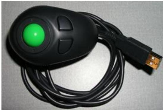
The hand held ball track mouse plugs into either of the USB ports on the back of the Ultimate Le. It fits nicely in either hand. It has three usable inputs, trigger (actuated with the index finger), ball to position the mouse arrow, right button depending on software.
